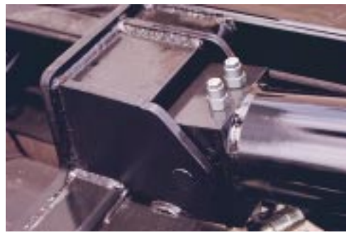
Dual Counter Balance Valves For Added Safety
