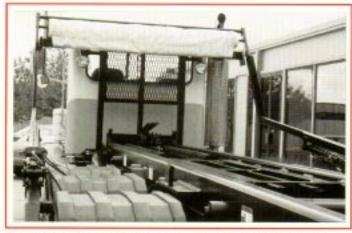
Extendable gantry to tightly fit 15 yard to 40 yard containers. Optional cab guard can be easily installed.
